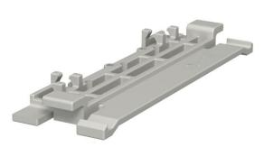
Cover clip for better and easier laying of lines in the WDK trunking. The cover fixing device can be moved along the entire length of the trunking. The cover clip is locked on one side and moved forward. This provides a 30° opening, meaning that cable routing is very simple. From trunking widths of 110 mm, the cover clips can also be used as a mounting aid.
